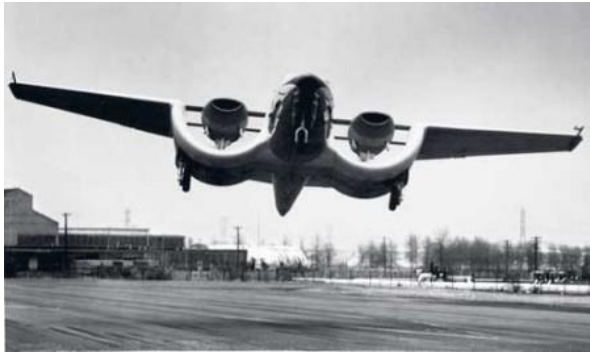
Figure 10: The Custer Channel Wing
