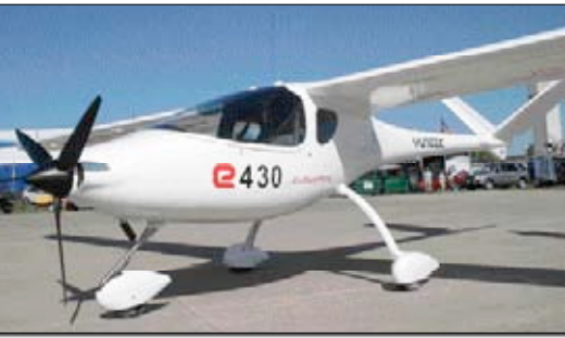
The Yuneec E430 from China appeared last June. It's LSA eligible, and may fly for 2.5 hours on a charge.
