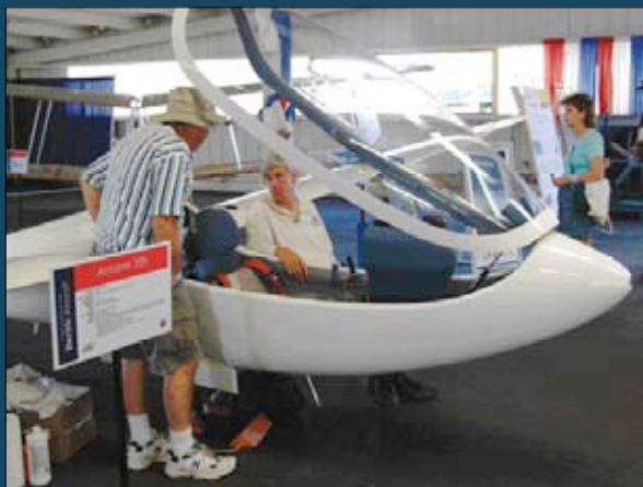
Dave Nader's 20-meter self-launching electric Antares sailplane is in commercial production in Germany.
